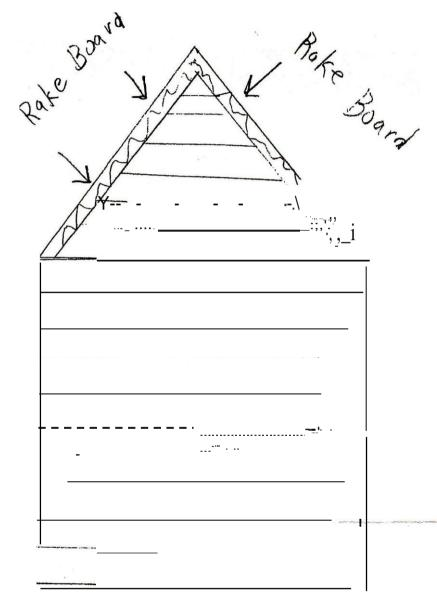
The rakeboard is a transition from the roof shingles to the siding. The rakeboard is covered with white metal. You may not install an antennae/dish on the siding and may not install through the roof shingles.
